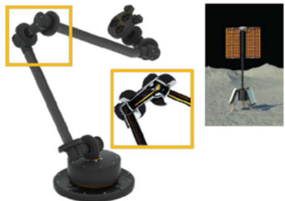
Figure 2 – LUnA Concept with Cutaway View (L) and SolarHub (R), which will adapt KSC EDS Technology
