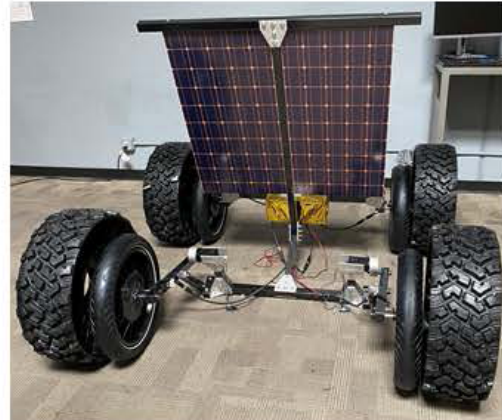
Figure 1- Maxar's Hybrid Iterative Testbed (HIT) for rover mobility technology evaluations.
